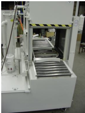
Double-Guillotine Door With Auto-Loader
