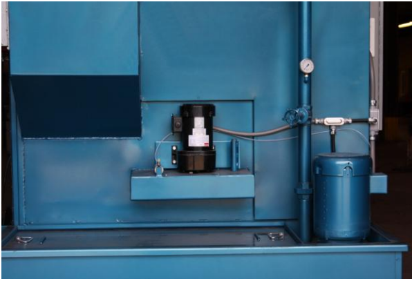
Back Side with Friction Drive Motor for Turn-Table and Large SS Screen Lid, Wash Pump.
