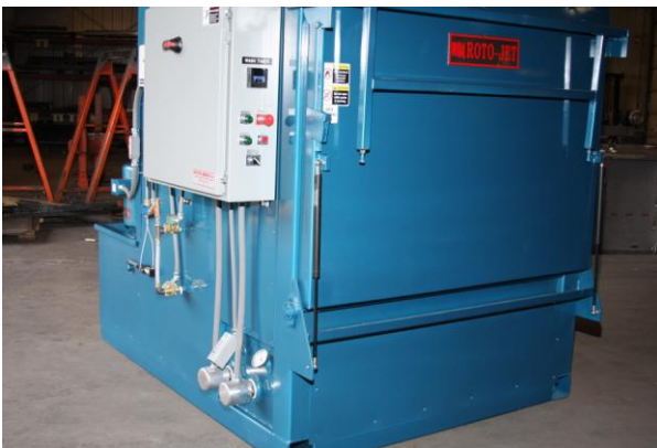
Front-Left Side showing Gas-Shock Door-Lift Springs. Handles swing down and out to provide door support. Industrial-grade electrical Panel with built-in Disconnect Switch.
