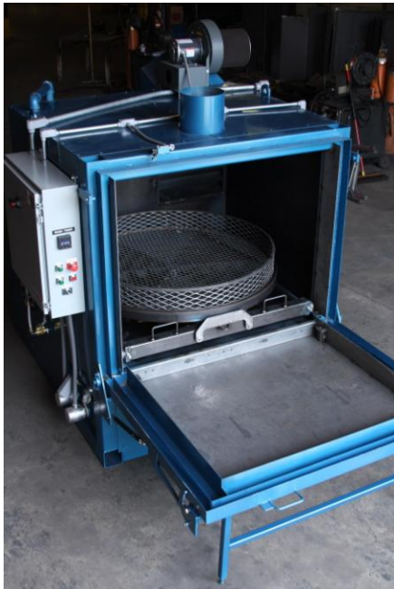
Basket and Carriage/Turntable Inside "Labyrinth" Door Sealing design reduces escaping vapor loss without rubber seals.
