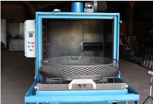
Front View Door Open with Basket, Turn-Table and Carriage on door.
