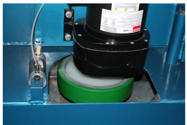
Friction-Driven Turntable with pneumatically operated tensioning cylinder. Turntable has manually-operated position-lock when on door for loading/unloading.
