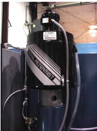
Exhaust Vapor-Mist Extractor
