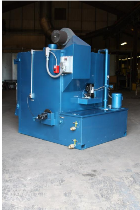
Right-Side showing HD Oil Skimmer, Hot-Air Blower, TT Compression Drive Mechanism, Overflow Valve, Drain Valve, Rinse-to-Drain Connection.
